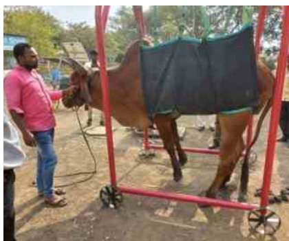
VNMKV developed Sick Animal Lifting Device
